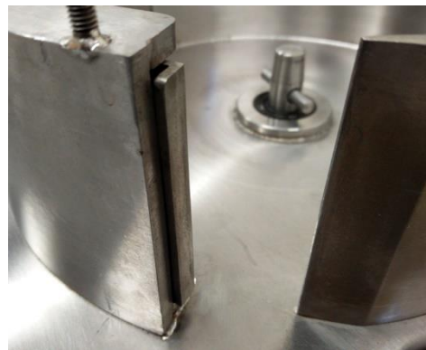
Figure 4: Incorrect plate seating
